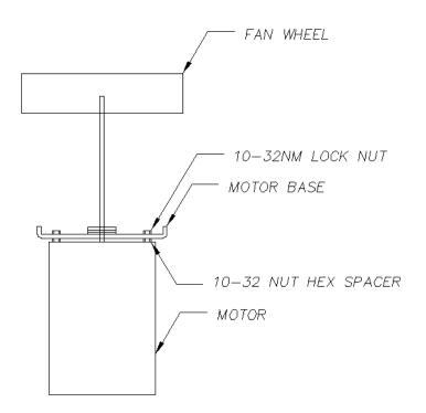
Step 14 There may be existing holes to use to mount the new motor to the oven. If not, Drill four (4) new 7/32" holes into the body to attach the new motor base after centering the motor in the collar opening. Attach the new base to the body with four (4) thread forming screws provided.
