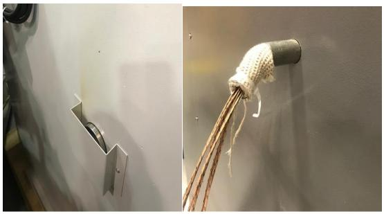
If the thermocouples must be routed through the door opening, they should enter the oven on the airflow return plenum side (suction side) at mid-height on the oven. The thermocouples should not be bundled at the point where they pass between the door and seal on the oven
