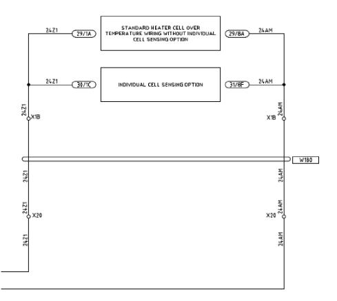
If the oven has the Individual Cell Sensing option, the over temperature switch inputs must be removed from the microcontrollers for the option.
