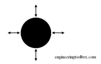
The black body is defined as a body that absorbs all radiation that falls on its surface. Actual black bodies don't exist in nature - though its characteristics are approximated by a hole in a box filled with highly absorptive material. The emission spectrum of such a black body was first fully described by Max Planck.
