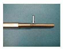
2. Use a piece of Scotch Brite pad to polish the surface of the shaft (at arrow) that will make contact with the bushing. If this surface is scarred and cannot be made smooth, replace the smart wave shaft.
