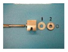
1. Remove smart wave from the solder pot and disassemble. Items 1 & 2 will no longer be used. Clean the shaft and bearing house.
