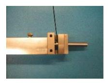
5. Reinstall the bearing house cover and attach the bearing houses and shaft to the main smart wave block. Turn the smart wave upside down and locate the ring adjustment. Move the ring adjustment as close to the bushings as possible and tighten the set screw. Reinstall the smart wave into the solder pot and flow the main solder wave to bring it to temperature. You should replace the carbon bushings every 2000 hours. Any questions please contact your nearest Vitronics Soltec office.
