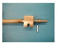
3. Insert the smart wave shaft through the bearing house. Slide the Ring Adjustment, Part number 7-424425 (at arrow), on the shaft with the chamfered side towards the wave area. Do not tighten the set screw.
