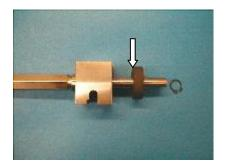
4. Slide the graphite bushing, part number 7-424424, on the shaft with the chamfered side towards the bearing house. Move the bushing completely into the bearing house and reinstall the "C" clip.
