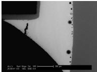
contamination on the metallization of component or board pads. In the early days this could typically be found at the surface of an immersion Ag finished pad (board suppliers have tackled this issue).
