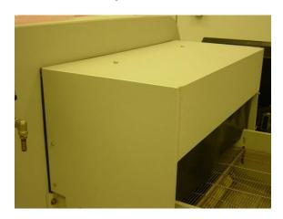
Load damper is located on the inside of the load end cover. There are two wing nuts inside the box. The damper moves horizontally into the machine.
