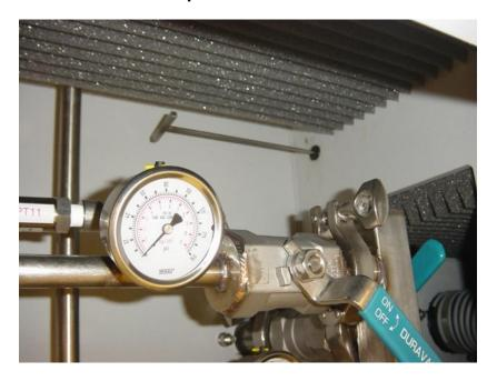
Damper rod is located insid the rinse section at the top of the machine. The damper is inside the exhaust duct and can not be seen. When the rod is pulled out, the exhaust is fully open, and when it is pushed in it is fully closed.
