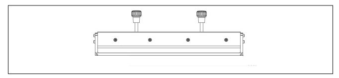
**1024009-xxx:** Is used on Edison printers only which utilizes the Quick Release feature. This assembly is like the blade assembly 1018140, with a higher deflection point of the squeegee blades. The blade holders have spring loaded floating side dams which keeps the paste roll with in the squeegee blade area, reducing bleed out on the outside of the blades. This blade assembly is comparable to the Accela style blade but the holder mounting is different.
