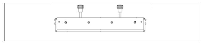
**2006150-xxx:** Currently the default blade assembly that's being shipped with the Edison series printers and will be used on Momentum II printers utilizing the Quick Release assembly. The blade holders have spring loaded floating side dams which keeps the paste roll with in the squeegee blade area, reducing bleed out on the outside of the blades. This assembly is like the blade assembly 1023036, with a lower deflection point of the squeegee blade.
