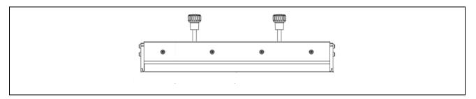
**1024142-xxx:** The blade holders are set to a 45-degree angle. Due to the 45-degree angle, these blades are for special applications. Can be used on Edison printers as well as the Momentum II printers utilizing the Quick Release feature. The blade holders have spring loaded floating side dams which keeps the paste roll with in the squeegee blade area, reducing bleed out on the outside of the blades.
