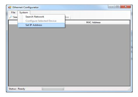
6. Enter the MAC Address found on the Ethernet communications card on the Protocol 3 control and the desired IP address for the control and click OK. (For example if you are connecting to a computer with an IP address of 192.168.10.1, subnet mask 255.255.255.1, you could set the control to 192.168.10.10).
